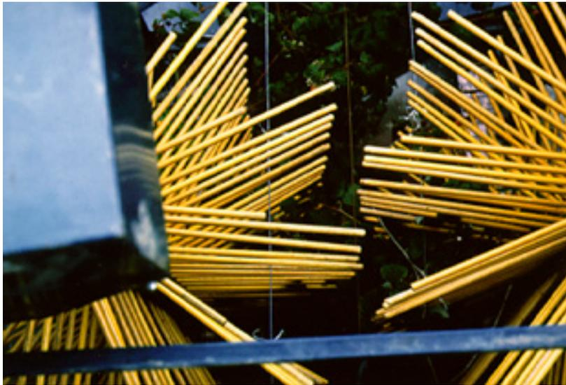
**Top side view from harvest machine, looking down on picking rods, which shake fruit from the row**
